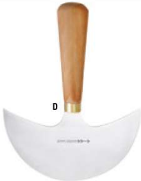
D PFEIL® HALFMOON KNIVES The traditional saddler's knife with a wide, semicircular blade allows the knife to be guided at a right angle even when cutting thick leather. Long, exact cuts are made with the middle of the blade, tight radii with the tips. Also used for thinning out leather. Ground ready to use. Handle made from oiled native cherrywood, with brass ferrule. Lifetime warranty on material and workmanship. 59-61 HRC. Blade width 125 mm No. 701366 150 mm No. 701367
