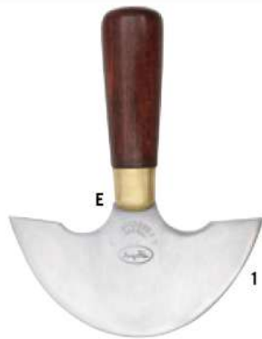
E OSBORNE SADDLER'S KNIVES Long, exact cuts are made with the middle of the blade, tight curves with the tips. Can also be used horizontally for thinning out and skiving leather. Ground ready to use. Red stained beech handle with brass ferrule. 55 HRC.
