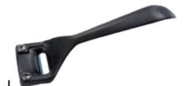
H STRAP CUTTERS FOR ENDLESS BELTS The strap cutter for endless belts allows you to easily and quickly cut leather straps. In order to perform this operation, you need to make a hole in the leather piece, through which the strap will be inserted. Then scrape along the edge of the hole until a piece of belt protrudes from the strap cutter. Now you can simply pull on the strap piece and the strap will cut itself around the hole edge until the leather piece is used up.
