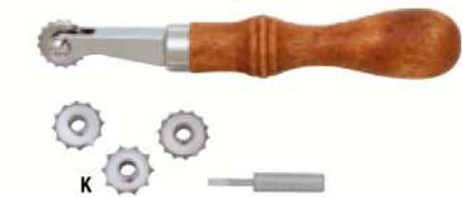
K STITCH MARKERS, 6-PIECE SET The stitch marker is used to mark the distance between the individual insertion holes of a stitch. The set contains four replaceable marking wheels with seam spacings of 3,5 mm, 4 mm, 5 mm, and 6 mm. Includes a small screwdriver to replace the wheels. Overall length 140 mm No. 708299
